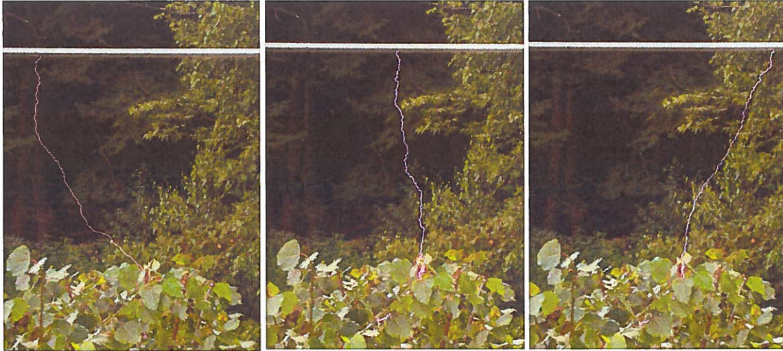
Figure 5-6 Flash overs to Vase, 230 kV, Vertical, Natural Vegetation
