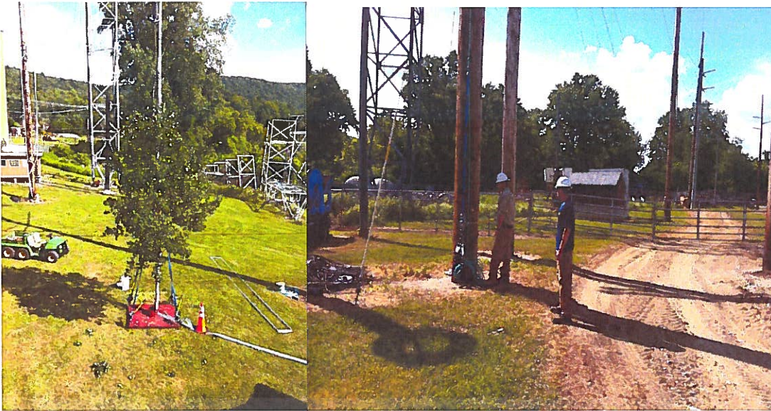
Figure 3-2 Photograph of test set up. Vertical clearance set using winch.
