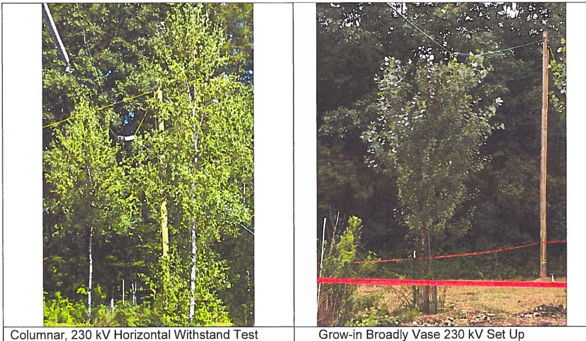
Figure 5-2 Views of switching impulse withstand test setups for natural trees.
