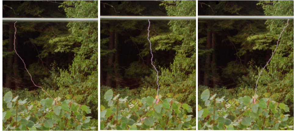
Figure 1-1 Flashovers to Vase, 230 kV, Vertical, Natural Vegetation
